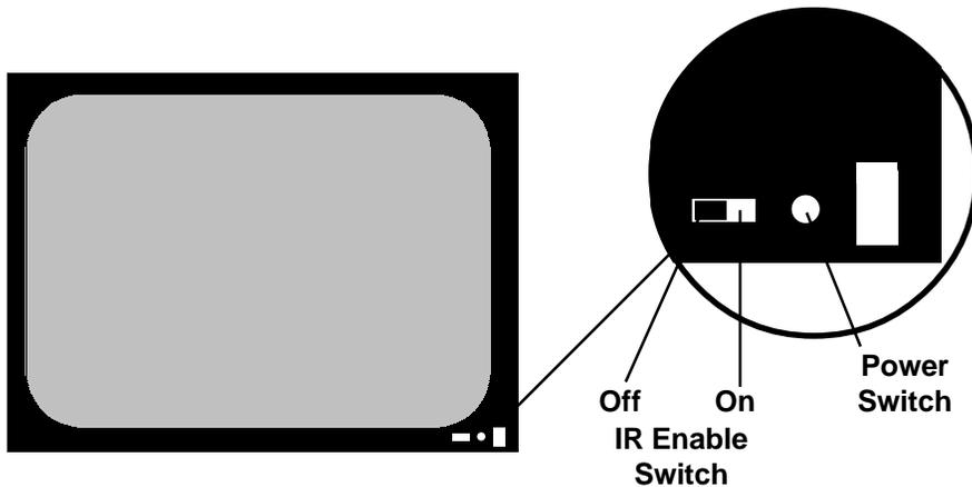
**Note:** Manual power switch is inactive with HARC option installed.
